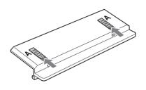
③ Insert the unit ejector (A) horizontally in the direction of the arrow until it clicks.
